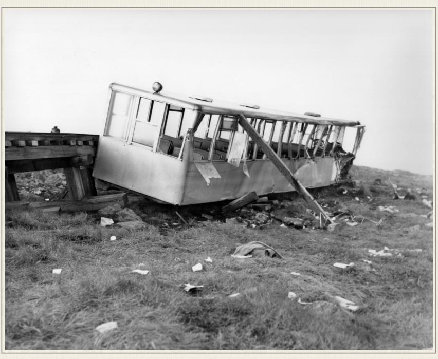
"It is apparent from the testimony taken from the involved persons that the switch was properly closed for main line use after the last train movement was made through the side track. It is also apparent that as engine No. 3 approached just prior to the derailment that one of the flip rails was in a position across the cog rack as it would be for a train movement to the side track.
