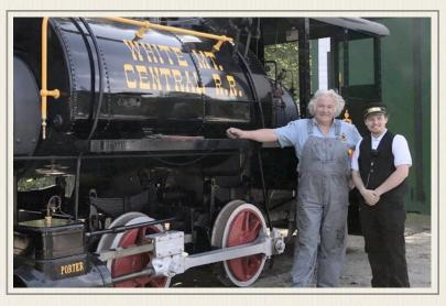
4-0 wheel arrangement. Originally owned by Koppers of Nashua, N.H., a creosote plant that creosoted railroad ties, telephone poles, and other wood products, the Porter started as a coal burner. It has operated as a wood burner since it was purchased by the WMCRR." - *NH DOT files / Moody email to Jitney Jr. - Mar 15, 2020 / North Conway, New Hampshire FB page - Sep 10, 2018*
