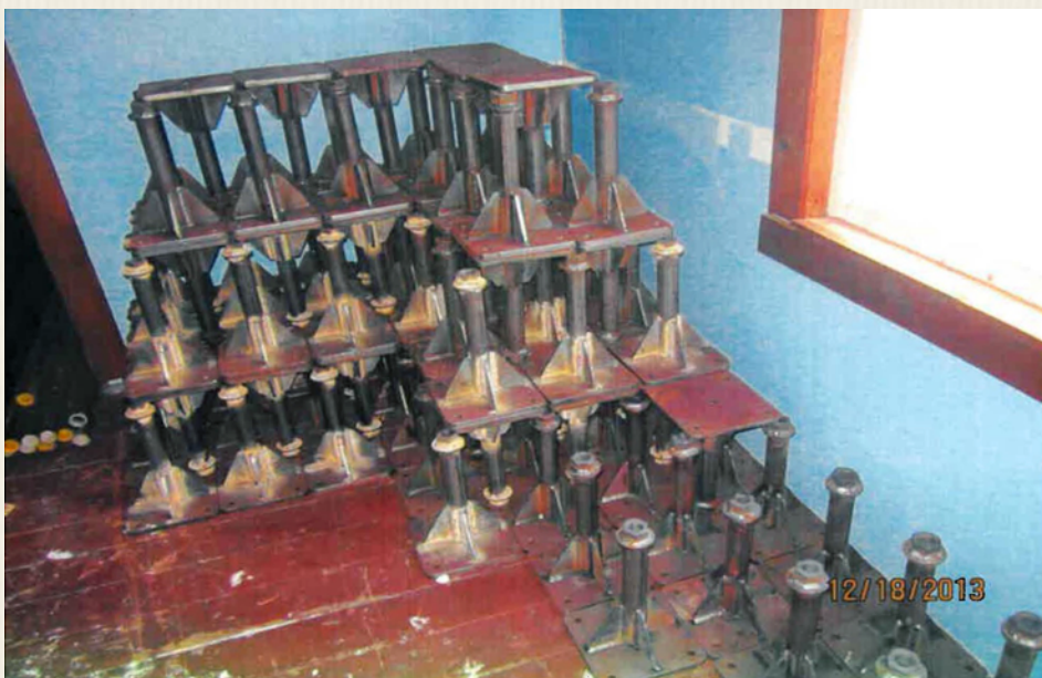
View of Some of the Fabricated Short Support Columns
