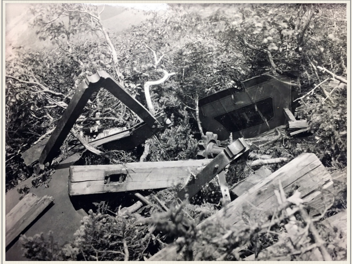
The broken frame, pinions, shaft and tender the scrub of Burt's Ravine (1929) NH Public Service Commission Peppersass Accident photo
