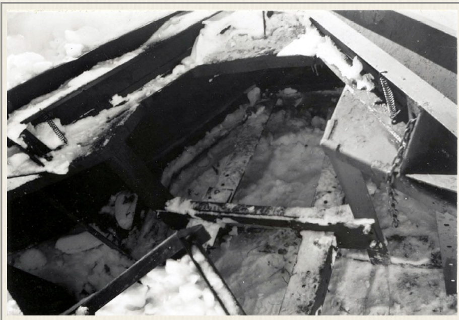
Close-up of mounting bracket of U.S. Forestry V-plow (Mar 1952) - Davenport-Besler photo
