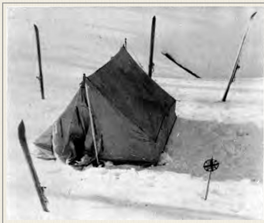
Primus Stove CO Test Tent pitched on snow. One of two low-walled 5x7 foot tent with sewn-in floor and sleeve type entrance allowing the tent to be closed tight while the stoves are operated. (1942) - Swarthmore University Collection
