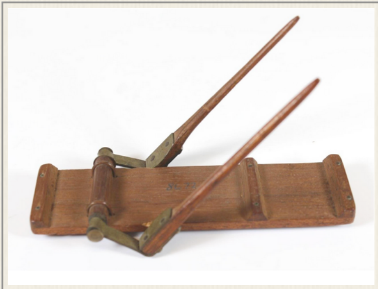
Model slide board (circa 1870) or "Devil's Shingle," used by workers on Mount Washington Cog Railway. Wooden board with three transverse wooden cleats on top surface. Bottom surface has longitudinal wooden cleat at front and one longitudinal brass track at rear (second track missing). Number "8672" written in ink on top surface. Tapered wooden brake arm on each side, attached to brass axle with brass connecting hardware. (Dimensions: H-3 W-2 L-5 inches) - Gift of the Manchester Historic Association to N.H. Historical Society
